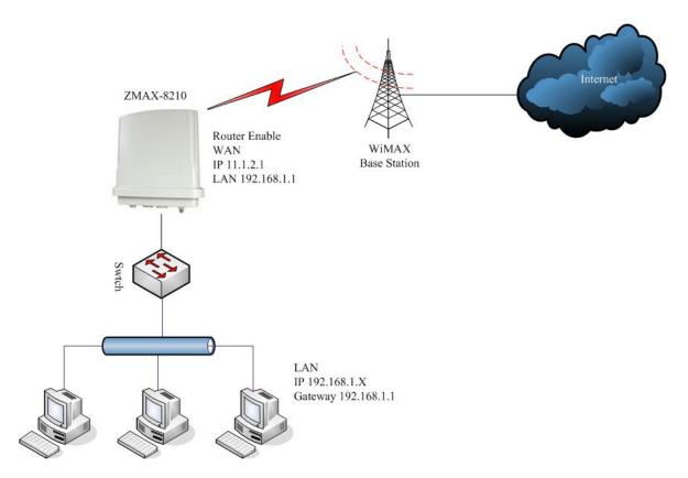
Figure 13 Wireless Router Mode
